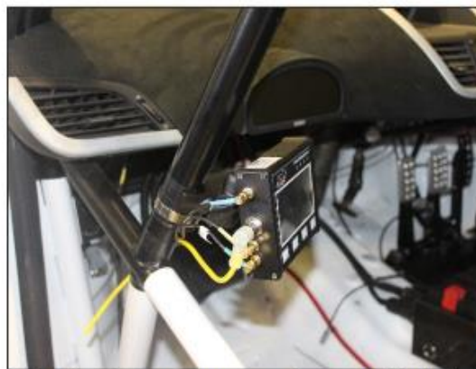
The RallySafe unit then mounts to the 25mm rubber ball mount (connected through the RallySafe connector).
