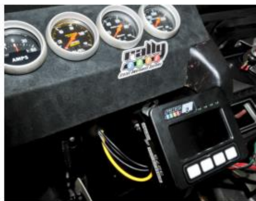
The RallySafe unit then mounts to the 25mm rubber ball mount (connected through the RallySafe connector).
